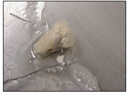
FIGURES 2 and 3. As for powders that are hydrophilic, a characteristic problem with them is the formation of lumps of product with a hydrated skin but a non-hydrated dry core. The particles on the inside become shielded by that skin, and thus they cannot interact as desired with the liquid
