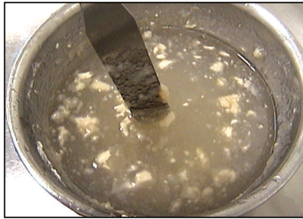
FIGURES 2 and 3. As for powders that are hydrophilic, a characteristic problem with them is the formation of lumps of product with a hydrated skin but a non-hydrated dry core. The particles on the inside become shielded by that skin, and thus they cannot interact as desired with the liquid
