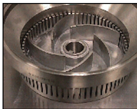
FIGURES 7 and 8. While high-shear mixing does not effectively mix difficult powders with liquid during in-tank mixing, the high-shear principle can be harnessed with good results for in-line blending
